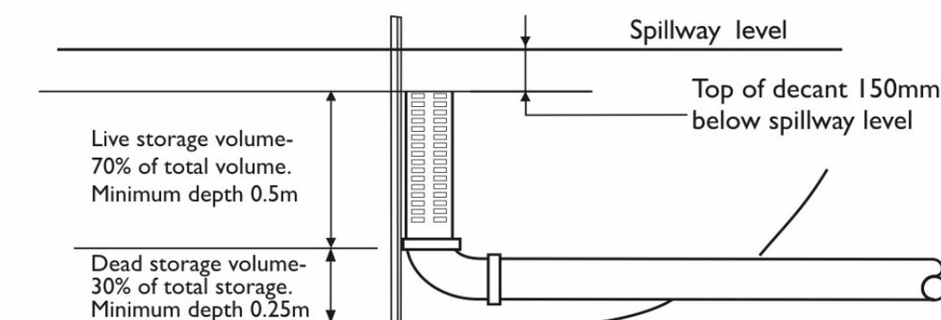
Build a one metre-wide trapezoidal spillway over the DEB embankment (preferably to spill to undisturbed land). The spillway must always be at the lowest point of the bund. It must be level across its width, 150 millimetres above the invert of the upstand and at least 250 millimetres deep. Stabilise the surface of the spillway against erosion if the downslope is more than 2 percent; for example, with needle-punched geotextile fabric, 150-300 millimetre-diameter rock or concrete.
